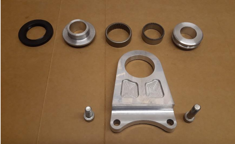
Below: Rear caliper assembly with needle roller bearing.
