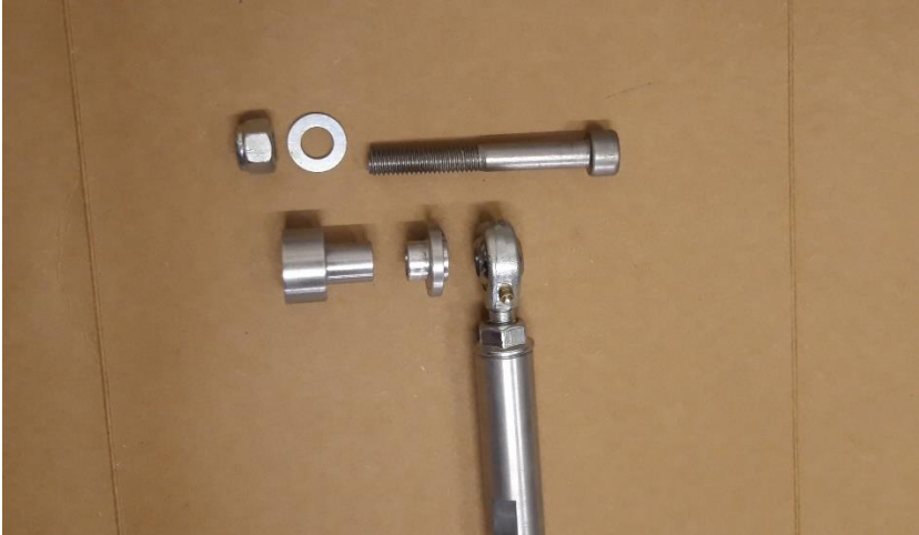
Below: brake arm rod – items for fitting to frame below right-hand foot peg. Fitted from indie the frame.
