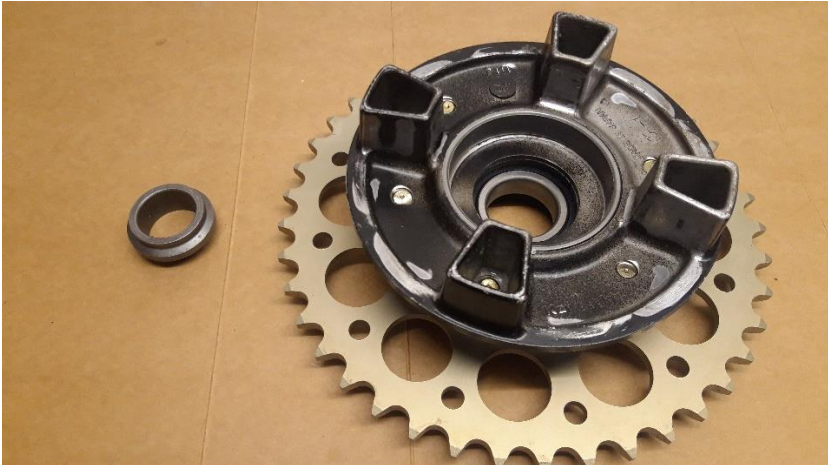
Below: Steel spacer for inside sprocket carrier.
