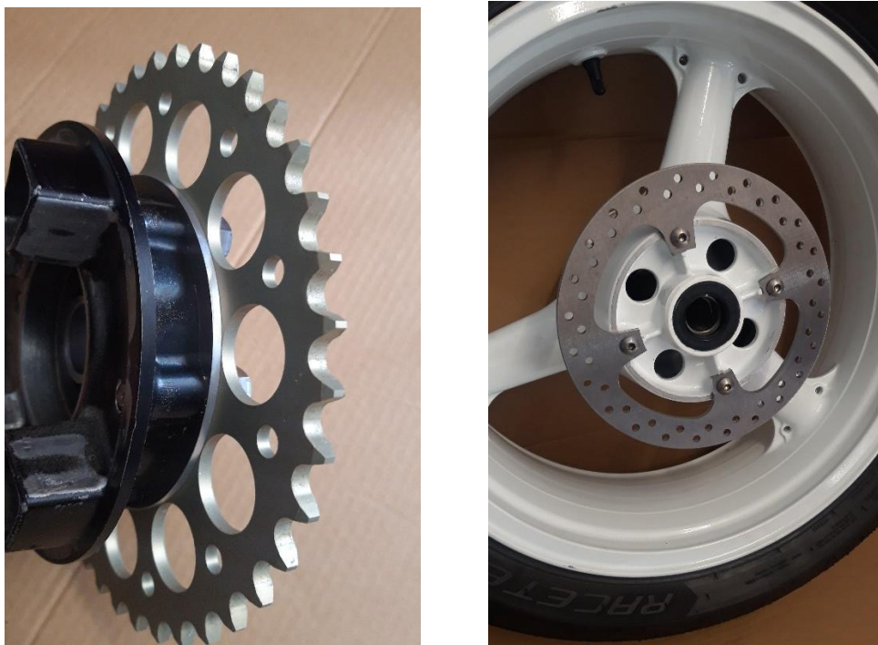
Below: sprocket with spacer for chain alignment fitted + rear disc fitted
